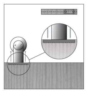
MAKE SURE TO DRILL THE PILOT HOLES CENTERED TO THE THICKNESS OF THE TOP OF THE DOOR
