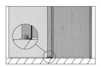
OPEN THE DOOR FULLY. THAT IS THE SIDE THAT THE FLOOR GUIDE WILL BE LOCATED.
